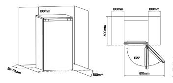
**Suggest:** It is advisable for there to be 50-70mm of space from the back to the wall, at least 100mm from its top, at least 100mm from its side to the wall and a clear space upfront to allow the doors to open 135°.As shown in follow diagrams.
